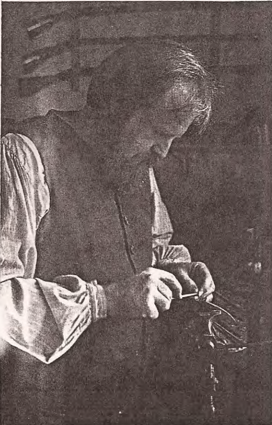
Gunsmith George Suiter patiently shapes a flintlock plate, a task requiring many hours of filing (above). He and Blair Taylor operate the rifling machine (opposite, top), which cuts spiral grooves in the rifle's smooth barrel. In the reconstructed Anderson Blacksmith Shop Richard Guthrie, Ken Schwartz, and Peter Ross (opposite, lower, front to rear) heat and work red hot iron in three of the shop's seven forges.
